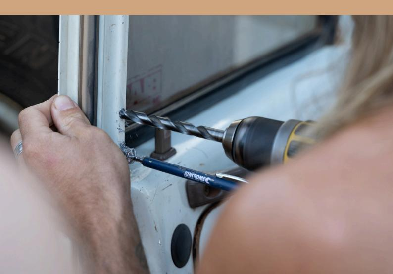
SPRAY SOME LANOLIN (OR SIMILAR) INTO THE DOOR FRAME TO PREVENT FUTURE CORROSION.
