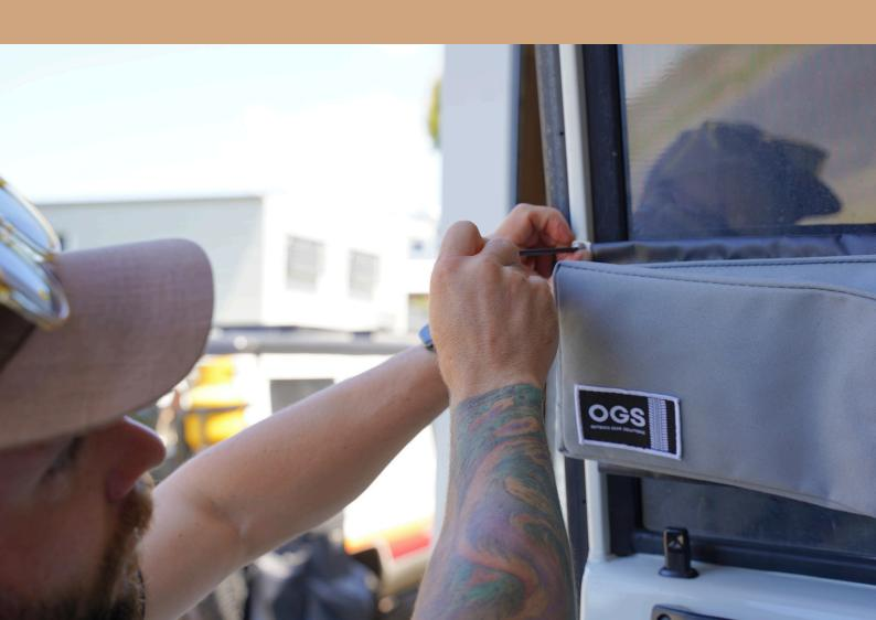
YOU CAN NOW THREAD THE LONGER MOUNTING WIRE THROUGH THE BOTTOM OF THE JOEY TO MARK THE CENTRES FOR DRILLING.
